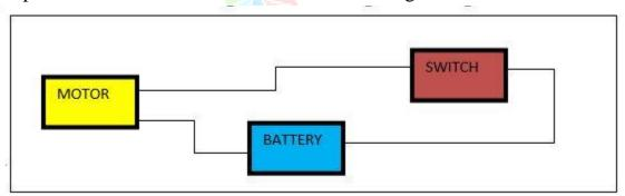
Step 11: Turn on the switch and see if hands are moving in correct direction, reverse the battery polarity if it is moving in opposite direction.
